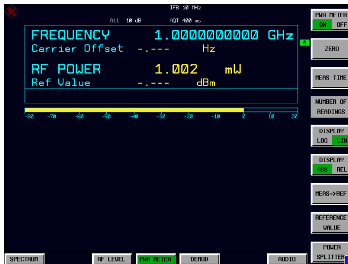
Fig.2-4 RF power measurement in UNIT Watt
