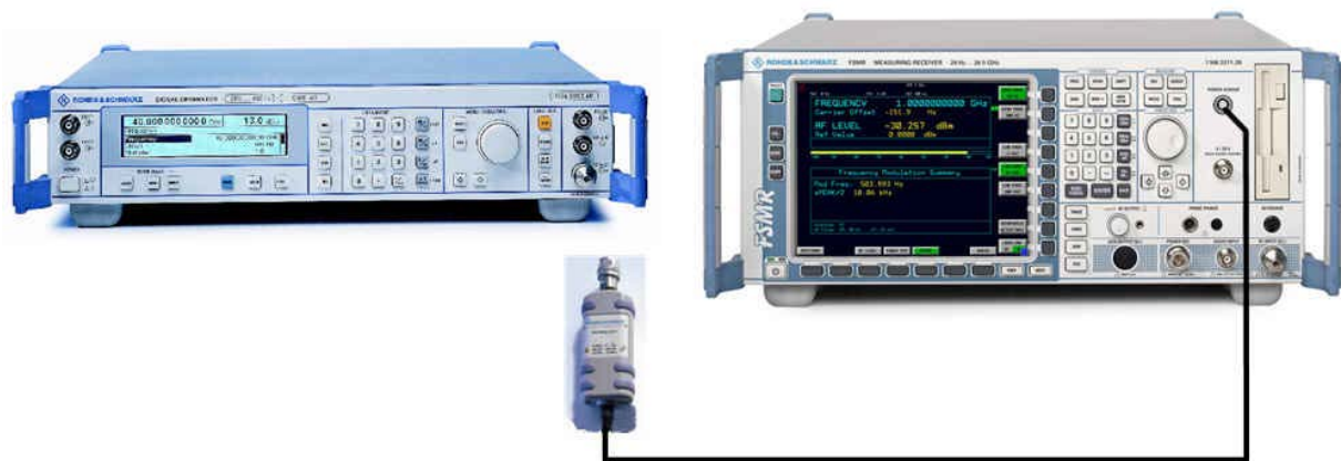
Fig.2-2 RF Power measurement setup
