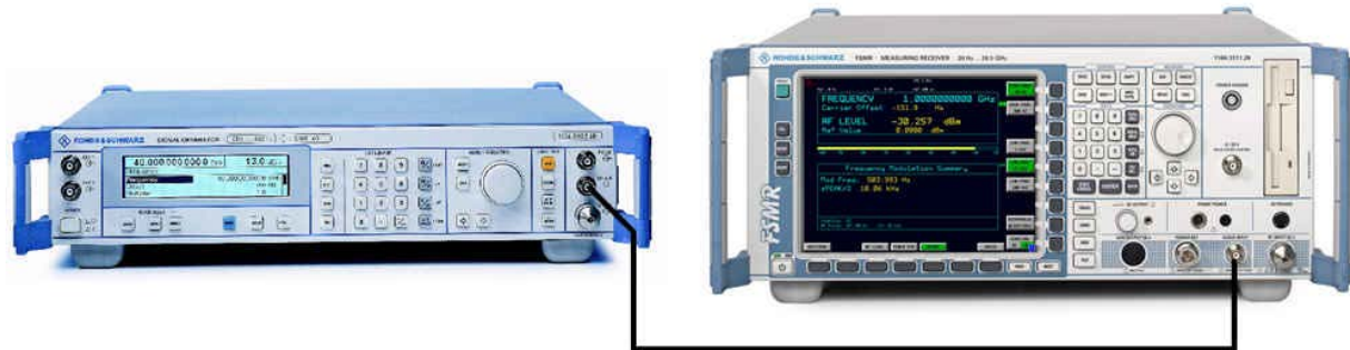
Fig.2-13 Audio measurement setup
